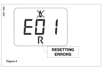
To RESET the gas boiler, turn selector (Figure 2) to "R" for at least 2 seconds. If the fault persists, call an authorised service centre.
