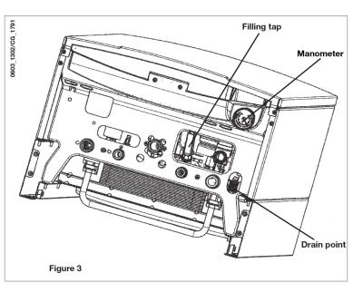
The boiler is supplied with a hydraulic pressure sensor, which blocks the boiler in case water is lacking.
